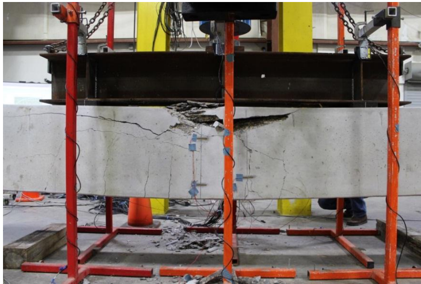
Figure 4.13 Failure mode in standard control (C-2).
