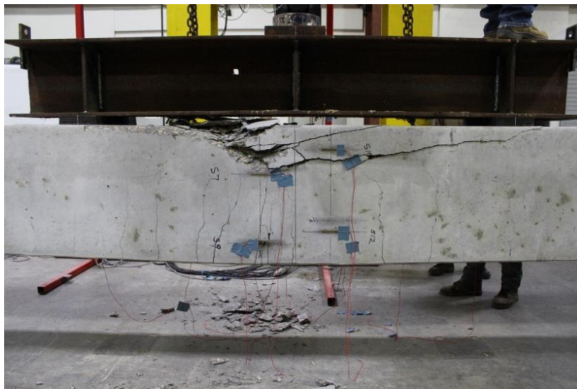
Figure 4.14 Failure mode in control with tight spiral layout (C-1).
