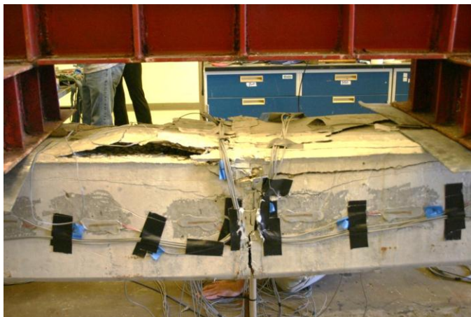
Figure 3.19 Ultimate stage of splice 2.
