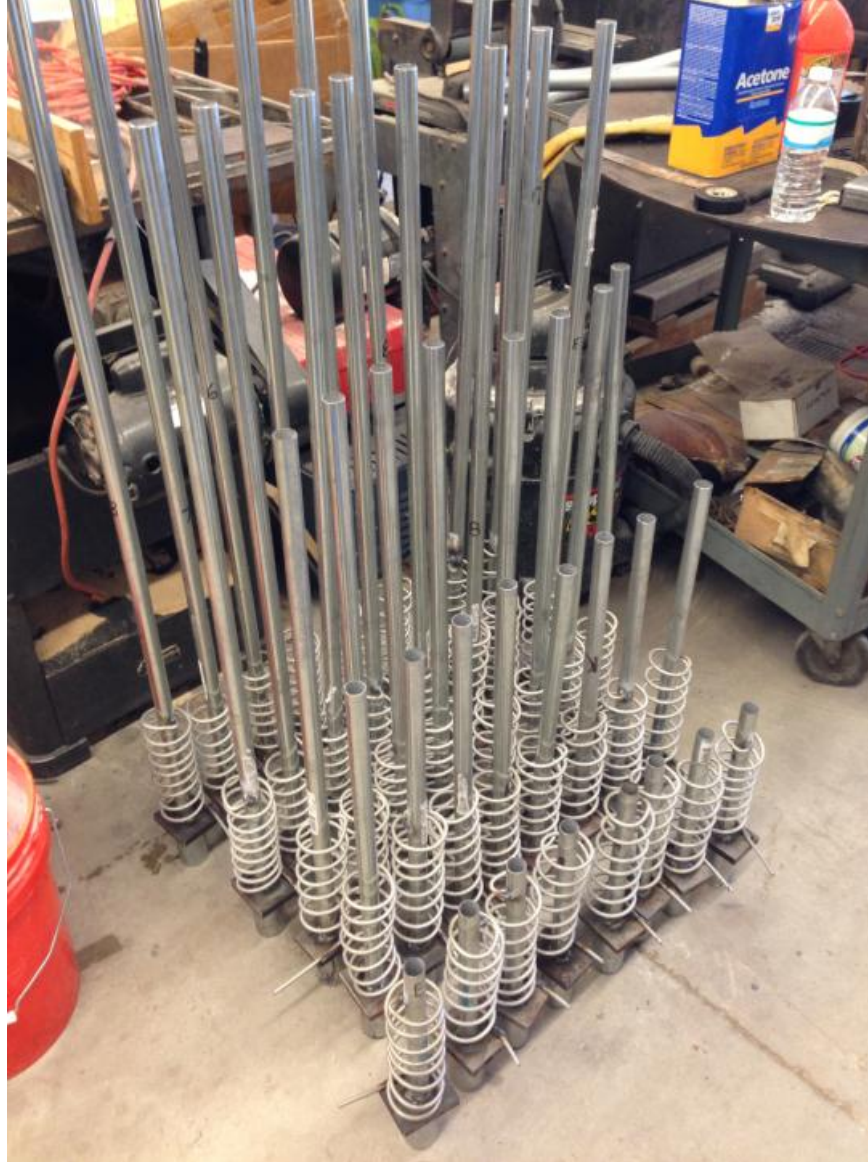
Figure 4.3 Finished internal splicing components.
